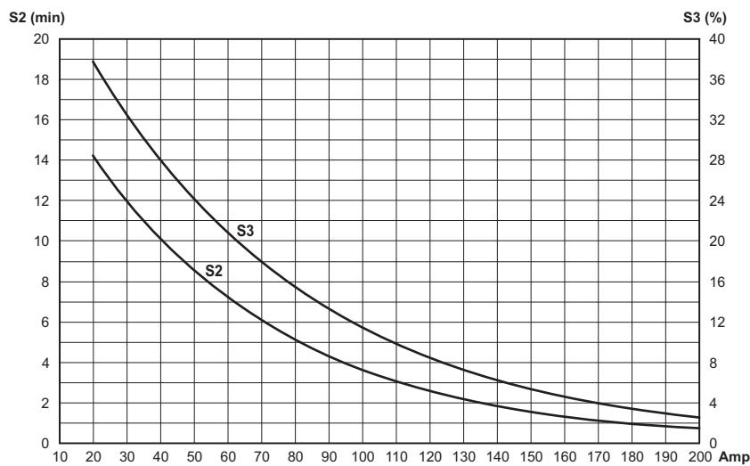
Motor with thermal switch
