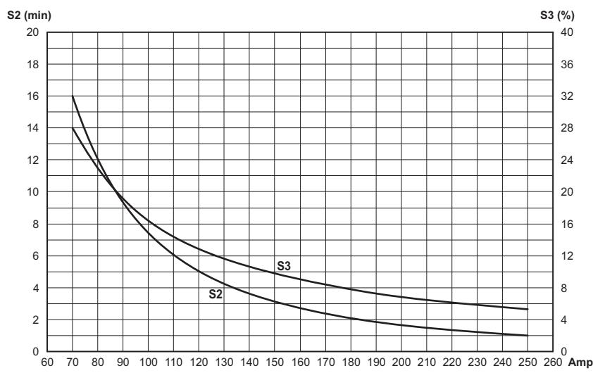
Motor with thermal switch
