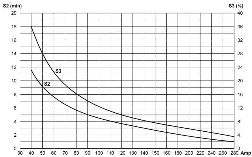
Motor with thermal switch
