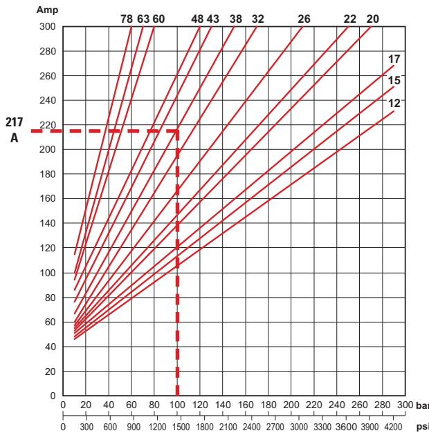
Taking again the current consumption on the S2-S3 diagram, you have a S2 duty equal to 1.55 (1'32") minutes and a S3 duty equal to 5.1 % (30 s on a cycle of 10 minutes).
