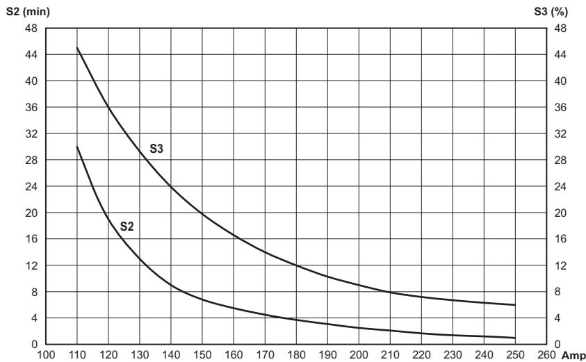
Motor with thermal switch
