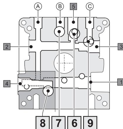
Optional flow control valves or plug on cavity 9
