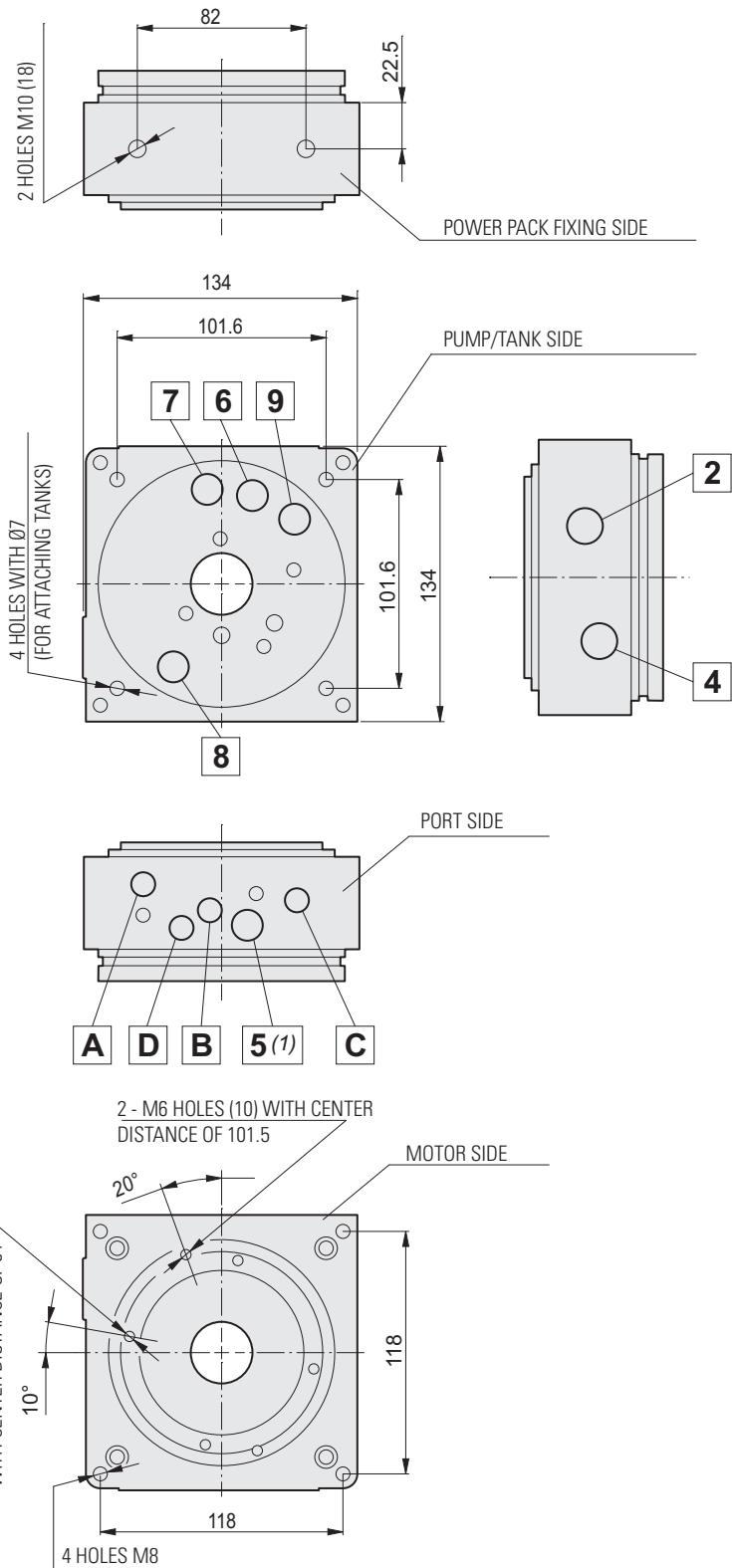
The cavities (1-2-3-4-5) and the ports (A-B-C) are marked on the die-cast endhead. The dimensions on the drawing are the same for all endhead.
