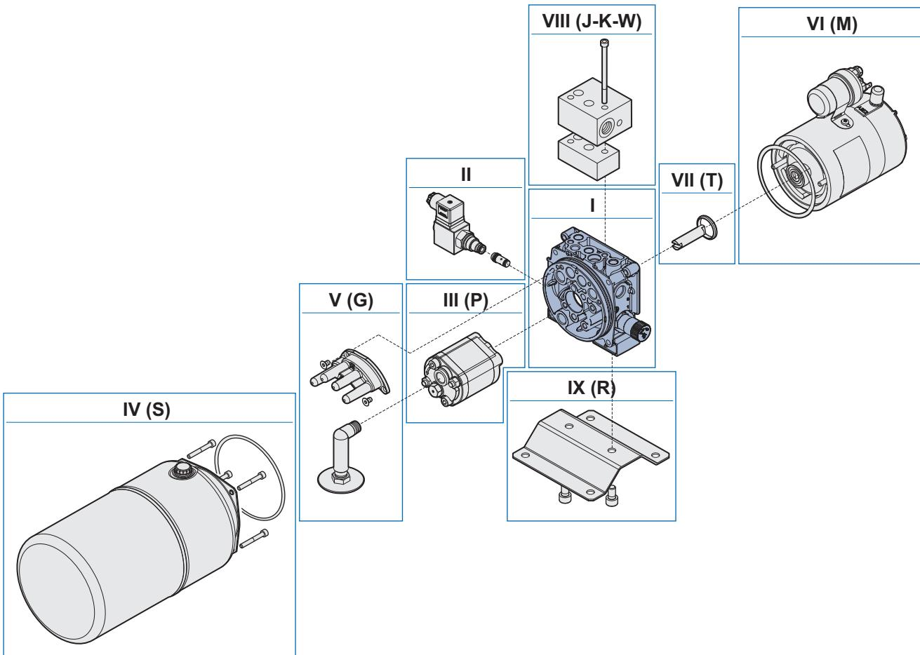
With its great modularity, the FP series of power packs can create multiple configurations which satisfy requirements in a wide range of applications. To make it easier to choose components, the power pack is subdivided into sections.
