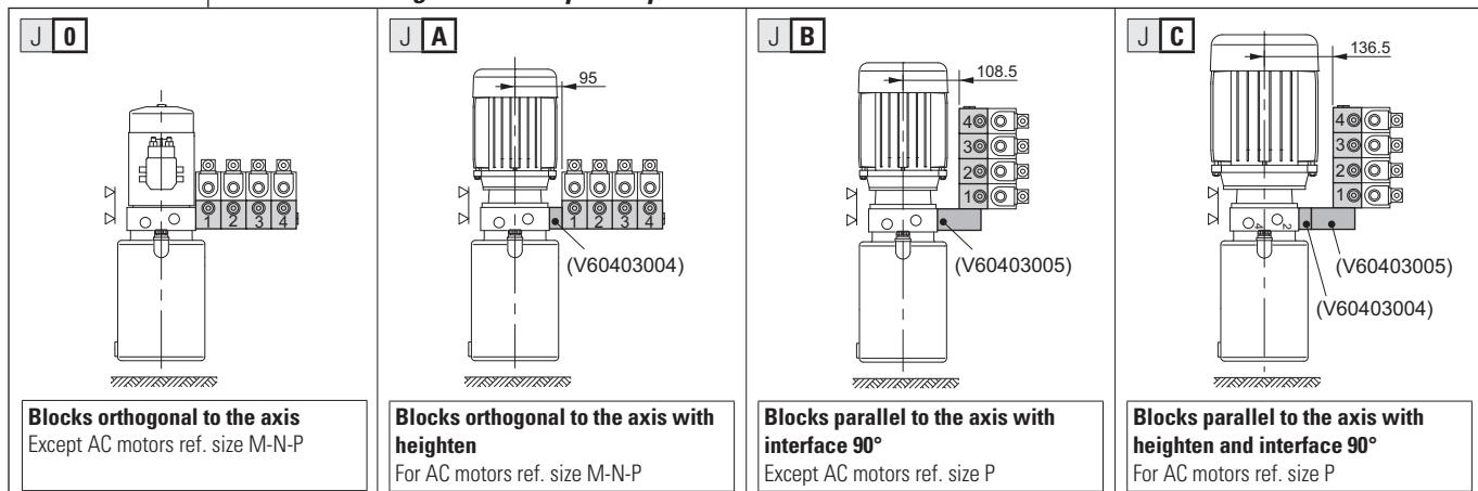
The blocks can not be mounted with motors oriented in position "1" - DC motors, see page 76. AC motors, see page 82.
