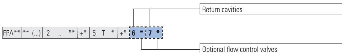
Return cavity, omit if not required flow control valves
