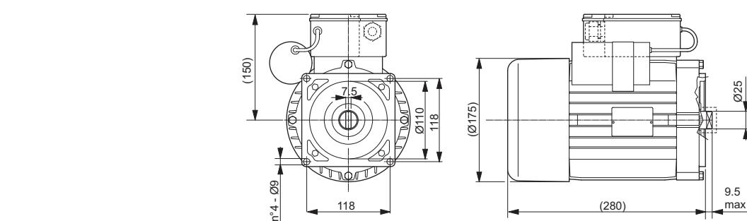
**Single-phase motors 4 Poles - 230 Vac 50Hz - Direct fixing**
