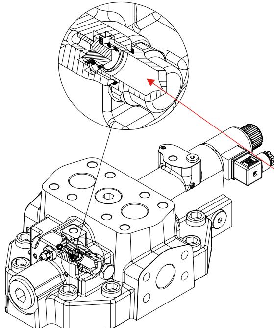
For closed circuit operation, the motors can be equipped with built in flushing valve.
