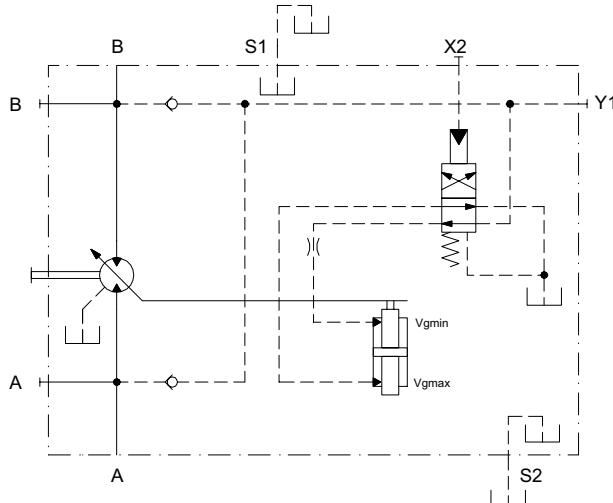
The hydraulic two positions control allows the displacement of the motor to be set to  $Vg_{max}$  or  $Vg_{min}$  by applying or not a pilot pressure at port X2. The feed back spring is missing so  $Vg_{max}$  or  $Vg_{min}$  only can be set. Minimum required pilot pressure = 10 bar [145 psi] and maximum permissible pressure at port X2=100 bar [1450 psi]. The swivel range is 1 (from  $Vg_{max}$  to  $Vg_{min}$ ) or 2 (swivel range from  $Vg_{min}$  to  $Vg_{max}$ ).
