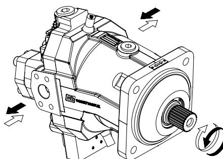
The hydraulic limiting device makes possible to reduce the pressure setting of RPE control by means of an external pilot pressure applied at port X2. The RPE control pressure setting is reduced proportionally to the pilot pressure in the ratio of 1/17 (for each pilot pressure bar, the preset operating pressure is reduced of 17 bar) [170 psi each 10 psi of pilot pressure]. Max permissible pilot pressure at port X2 = 100 bar [1450 psi].
