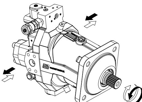
The RID control version with the pressure override allows the motor to swivel to  $Vg_{max}$  when the pressure setting is reached. Same as RIN control, the motor displacement is adjusted to  $Vg_{min}$  when the pilot pressure applied at port X2. If the operating pressure rises beyond the pressure setting, the pressure limiting device the motor swivels out to  $Vg_{max}$ . Swivel range is from  $Vg_{max}$  to  $Vg_{min}$  (displacement setting 1 per our ordering code).
