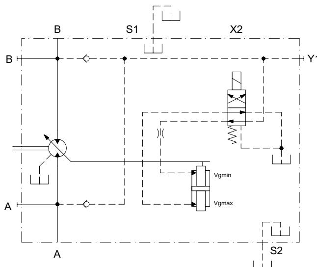
The electric two positions control allows the displacement of the motor to be set to  $Vg_{max}$  or  $Vg_{min}$  by switching an ON/OFF solenoid valve. The feed back spring is missing so  $Vg_{max}$  or  $Vg_{min}$  only can be set. 12V DC and 24V DC ON/OFF solenoid are available. The swivel range is 1 (from  $Vg_{max}$  to  $Vg_{min}$ ) or 2 (swivel range from  $Vg_{min}$  to  $Vg_{max}$ ).
