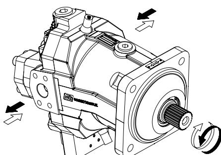
The "ROE" control allows a larger pressure range for displacement variation in comparison to "RPE" control. The increase of pressure range for variation from  $Vg_{min}$  to  $Vg_{max}$  allows a smoother working of the motor during displacement variation. The "ROE" allows the displacement variation with the pressure range show in the table.
