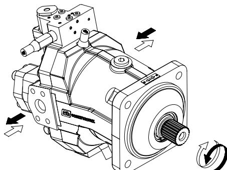
The RIE control version with the pressure override allows the motor to swivel to  $Vg_{max}$  when the pressure setting is reached. Same as RIN control, the motor displacement is adjusted to  $Vg_{min}$  when the pilot pressure applied at port X2. If the operating pressure rises beyond the pressure setting, the pressure limiting device makes the motor swivel to  $Vg_{max}$ . Swivel range is from  $Vg_{max}$  to  $Vg_{min}$  (displacement setting 1 per our ordering code).
