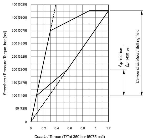
**Warning:** in case of displacement limitation, the control shall vary of a reduced  $\Delta p$  with respect to its standard one. Please contact Dana Brevini for more info.
