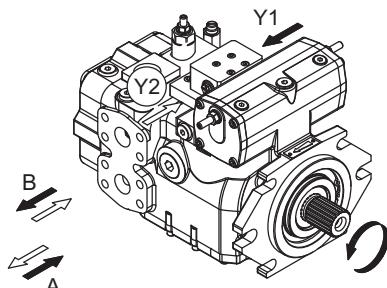
**Flow direction:** Correlation between direction of rotation (shaft view) control and direction of flow.
