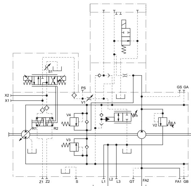
The electric cut-off valve, directly flangeable on S6CV pump housing, swivels back to zero the pump flow when power supply to the ON/OFF solenoid is cut-off. This valve has been designed for applications subject to safety rules, which required stopping of the machine in case of no electric signal. Feed voltage is 24V d.c. (optional 12V d.c.).
