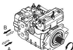
The displacement of the pump is directly proportional to the angle of rotation of the lever. The feedback system feels the position of the swashplate and works automatically to compensate for a positioning error. The diagram below shows the relationship between angle and displacement.
