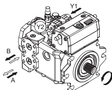
The pump displacement is proportional to the pilot pressure on Y1 or Y2 ports, which also affect flow direction. The feedback system feels the position of the swashplate and works automatically to compensate for a positioning error. Piloting can be provided by boost pressure from GS port. The piloting pressure will then have to be controlled by a joystick or by a pressure reducing valve (not supplied).
