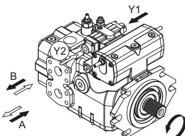
The pump displacement is proportional to the pilot pressure on Y1 or Y2 ports, which also affect flow direction. The feedback system feels the position of the swashplate and works automatically to compensate for a positioning error. Piloting can be provided by boost pressure from GS port. The piloting pressure will then have to be controlled by a joystick or by a pressure reducing valve (not supplied).
