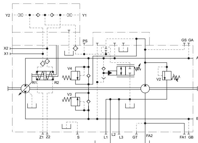
Pilot pressure = 6÷14 bar [87÷203 psi](at ports Y1, Y2)
