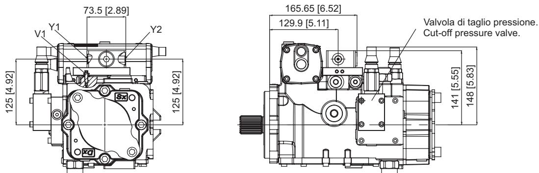
Y1-Y2: Attacchi pilotaggio comando / control piloting pressure ports - 1/4 G (BSPP) (ISO)
