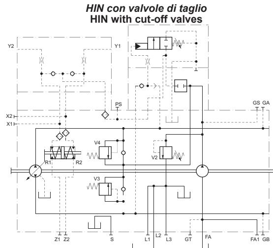
Pilot pressure = 6+14 bar [87+203 psi] (at ports Y1, Y2)
