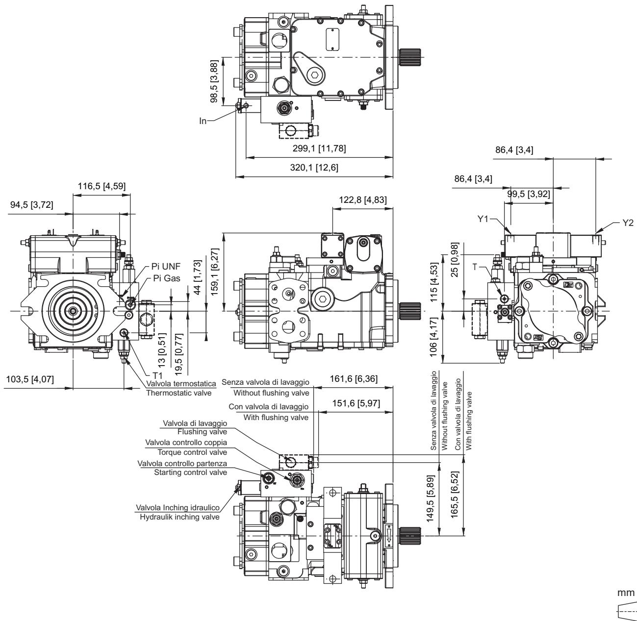
Y1-Y2: Attacchi pilotaggio comando / Control piloting pressure ports - 1/4 G (BSPP) (ISO)
