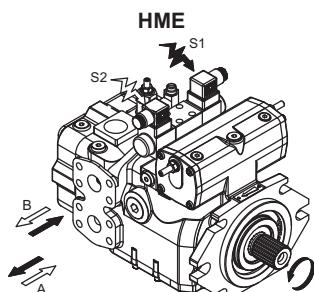
The "AUTOMOTIVE" (speed related) control, is used in hydrostatic transmissions with closed loop variable displacement pumps.
