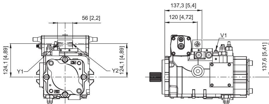
Y1-Y2: Attacchi pilotaggio comando / control piloting pressure ports - 1/4 G (BSPP) (ISO)
