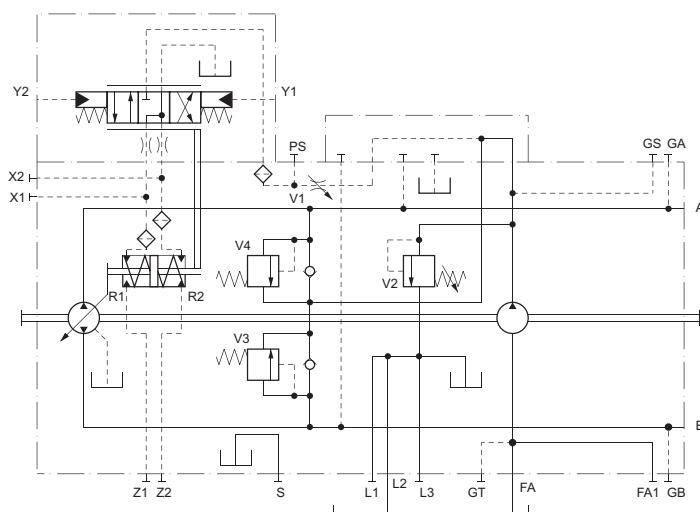
Pilot pressure = 6÷18 bar [87÷261 psi](at ports Y1, Y2)
