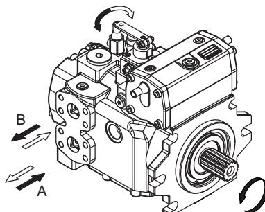
The displacement of the pump is directly proportional to the angle of rotation of the lever. The feedback system feels the position of the swashplate and works automatically to compensate for a positioning error. The diagram below shows the relationship between angle and displacement.
