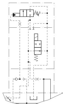
The electric cut-off valve, directly flangeable on S6CV pump housing, swivels back to zero the pump flow when power supply to the ON/OFF solenoid is cut-off. This valve has been designed for applications subject to safety rules, which required stopping of the machine in case of no electric signal. Feed voltage is 24V d.c. (optional 12V d.c.).
