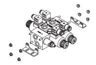
Intel module FE10, outlet module FU, mounting on BOTTOM position (standard mounting)
