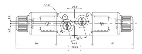
Fittings, max. tightening torque 60 Nm
