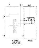
Outlet module FUS3 includes an overcenter valve to control the movement of a cylinder end connected to port A1.
