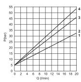
1 = 0.50 bar -2 = 35.90 bar -3 = 75.190 bar -4 = 160.290 bar Fluid used: mineral based oil with viscosity 46 mm²/s at 40°C.
