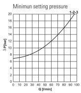
$1 = \max 50 - \text{bar} - 2 = \max 140 \text{ bar} - 3 = \max 350 \text{ bar}$ Fluid used: mineral based oil with viscosity 46 mm<sup>2</sup>/s at 40°C.
