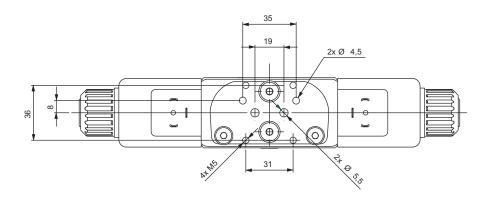
Fittings, max. tightening torque 60 Nm
