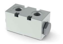
CM3P type modular check bankable valves allow one way free flow by raising a conical shutter, while in the opposite direction the fluid can return by means of a small piston piloted by the pressure in the other line.
