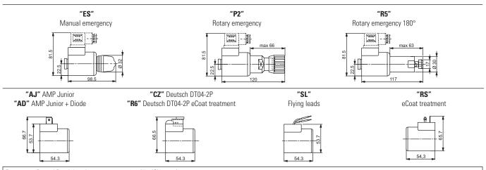
Emergency P2 and P5, tightening torque max.  $6 \div 9 \ Nm$  (CH n. 22)
