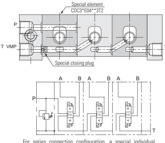
For series connection configuration, a special individual valve bank section (CDC3\*E04\*\*3T2) must always be used as first element (see ordering code page 25).
