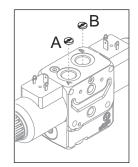
Interchangeable holed washer into fittings ports
