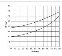
Pressure drops with compensator setting at 10 and 19 bar
