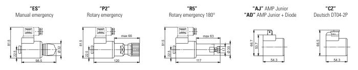
Emergency P2 and P5, tightening torque max. 6÷9 Nm (CH n. 22)
