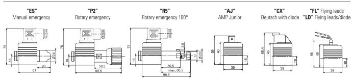
Emergency P2 and P5, tightening torque max. 6÷9 Nm (CH n. 22)
