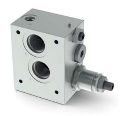
Closed center inlet module units FEH30LS for variable displacement Load Sensing pumps with pressure relief valve CMP30 and a pressure compensated load sensing signal bleed to minimize system losses even at high operating pressures. Signal bleed can be closed in case it is not required.
