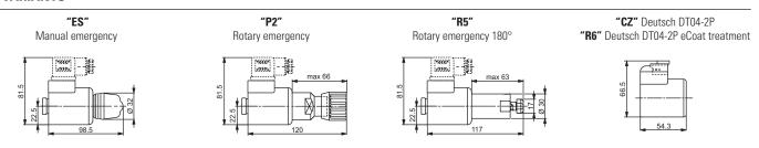
Emergency P2 and P5, tightening torque max. 6÷9 Nm (CH n. 22)
