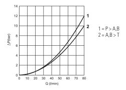
The diagram at the side shows the pressure drop curves for spools during normal usage.
