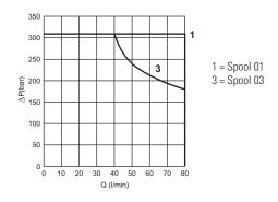
The tests have been carried out with solenoids at operating temperature and a voltage 10% less than rated voltage with a fluid temperature of 50  $^{\circ}$ . The fluid used was a mineral oil with a viscosity of 46 mm²/s at 40 degrees C.
