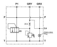
Module units FE02Q with pressure compensator for fixed displacement pumps and CMP-MC/MS adjustable pressure relief valve on LS line
