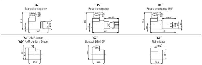
Emergency P2 and P5, tightening torque max. 6÷9 Nm (CH n. 22)
