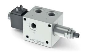
Inlet module units FE10PS with side ports, CMP10 adjustable pressure relief valve and electrical venting valve CRP0418NA normally open supplied with emergency control.
