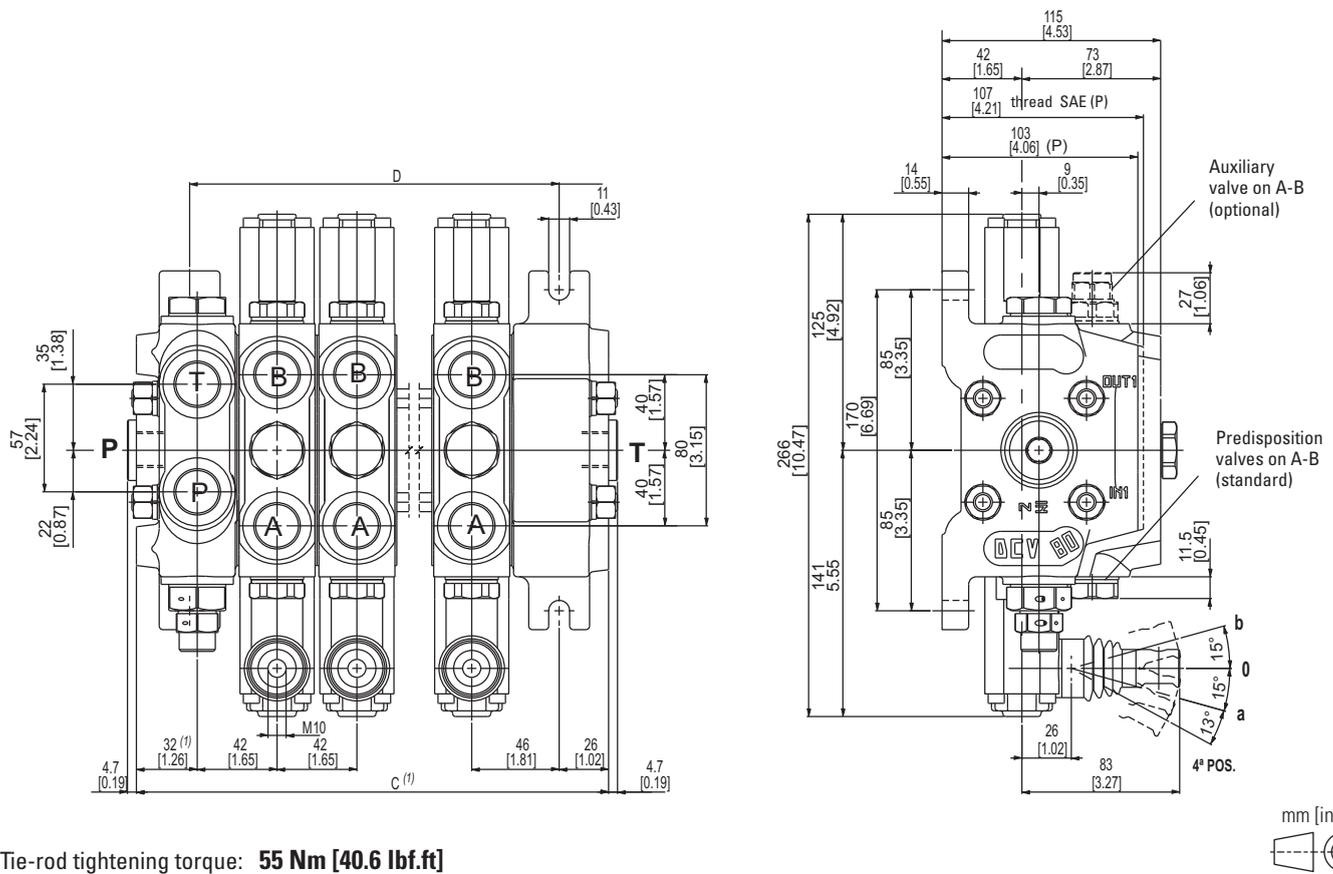
Tie-rod tightening torque: **55 Nm [40.6 lbf.ft]**
